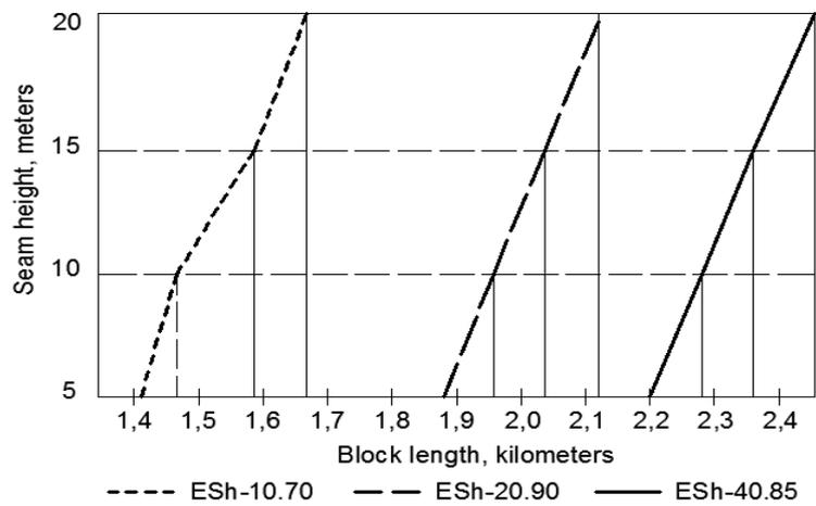
**Figure 3: The graph of the dependence of the excavator unit length for most common models of single-bucket walking dragline excavators involved in the transportless technological schemes of the carbonate deposits development.**
