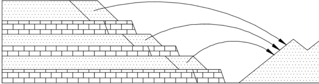
**Figure 1: Conventional geological section of formation of three horizontal layers of carbonate rocks, rocked off with the storage of overburden rocks in the inner dumps.**
