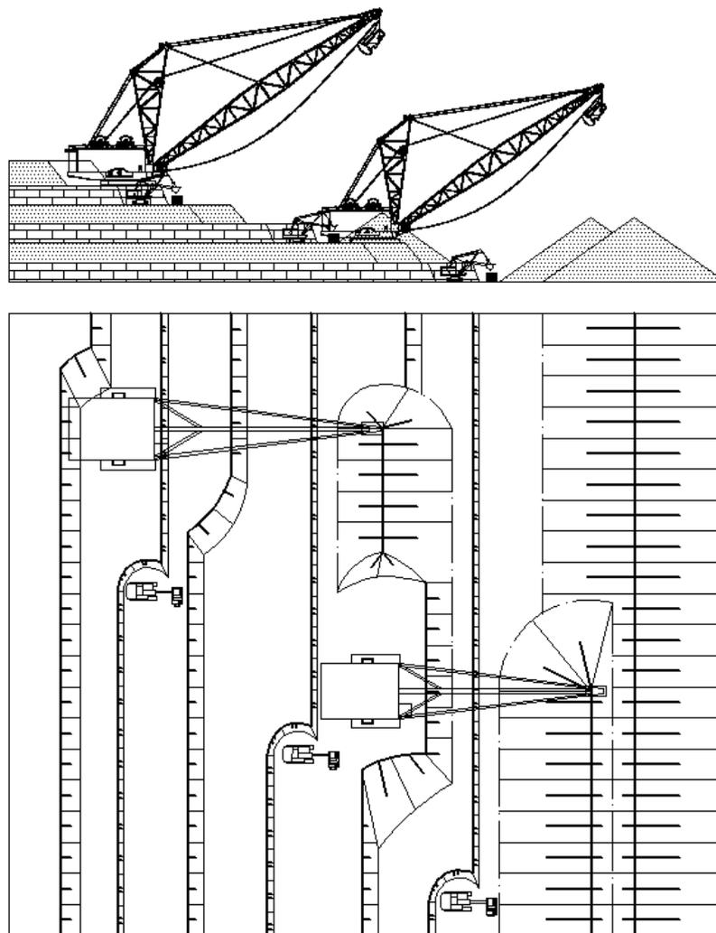
**Figure 2: Transportless mining system in developing the suite of three horizontal seams carbonate rocks.**
