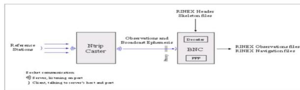
**Figure 1: Conversion of RTCM streams into RINEX files.**
