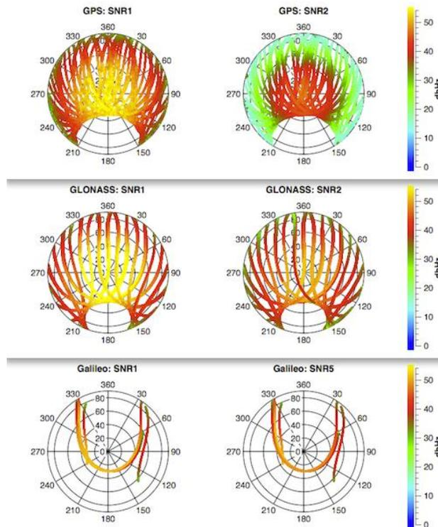
**Figure 5: Signal-to-noise ratio sky plots.**
