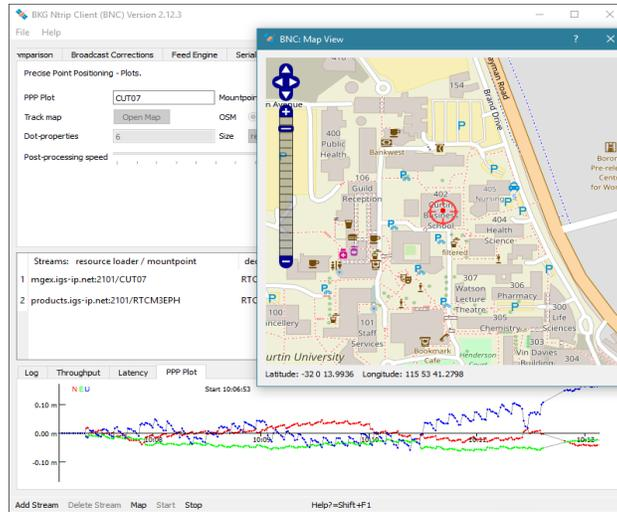
**Figure: 6. Tracking positions from BNC with Open Street Maps.**
