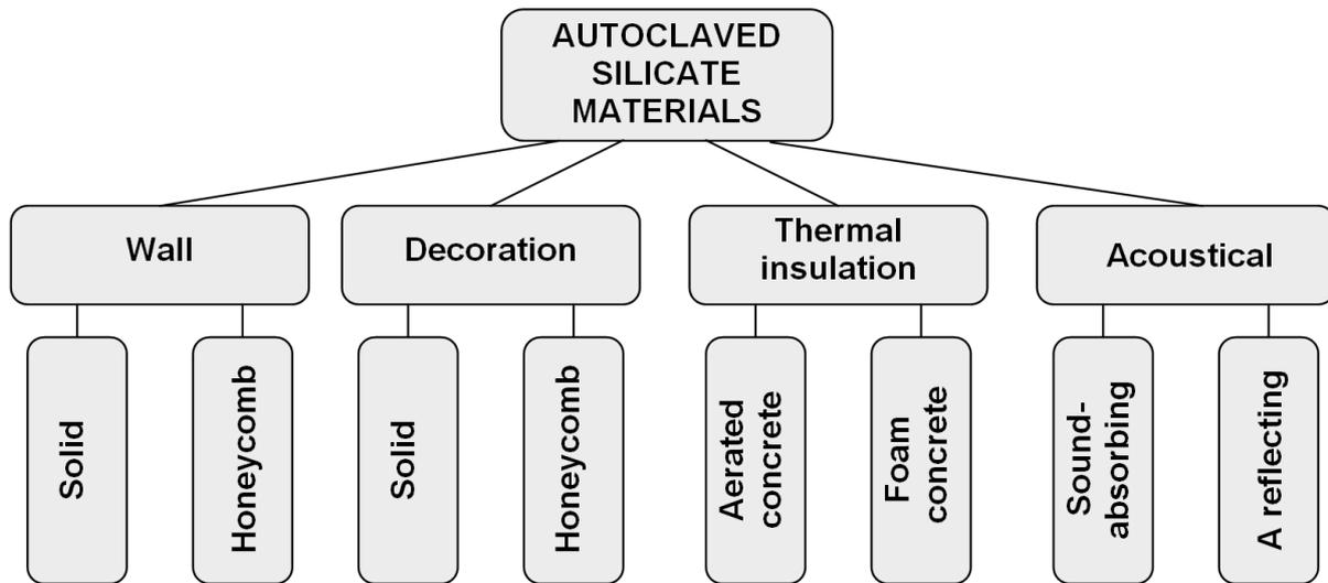
**Fig. 1.** Classification of autoclave silicate materials.
