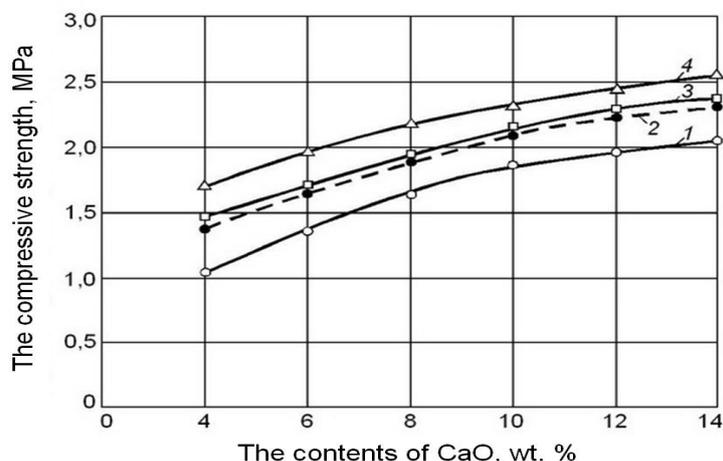
**Fig. 4.** The effect of lime content on raw material strength. Rock: 1, 2 - sandy loam; 3 - loam number 1; 4 - loam number 2; Binder: 1, 3, 4 - lime; 2 - LSCB
