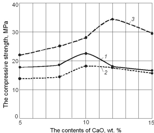
**Fig. 5.** The compressive strength limit of the samples according to lime content:
