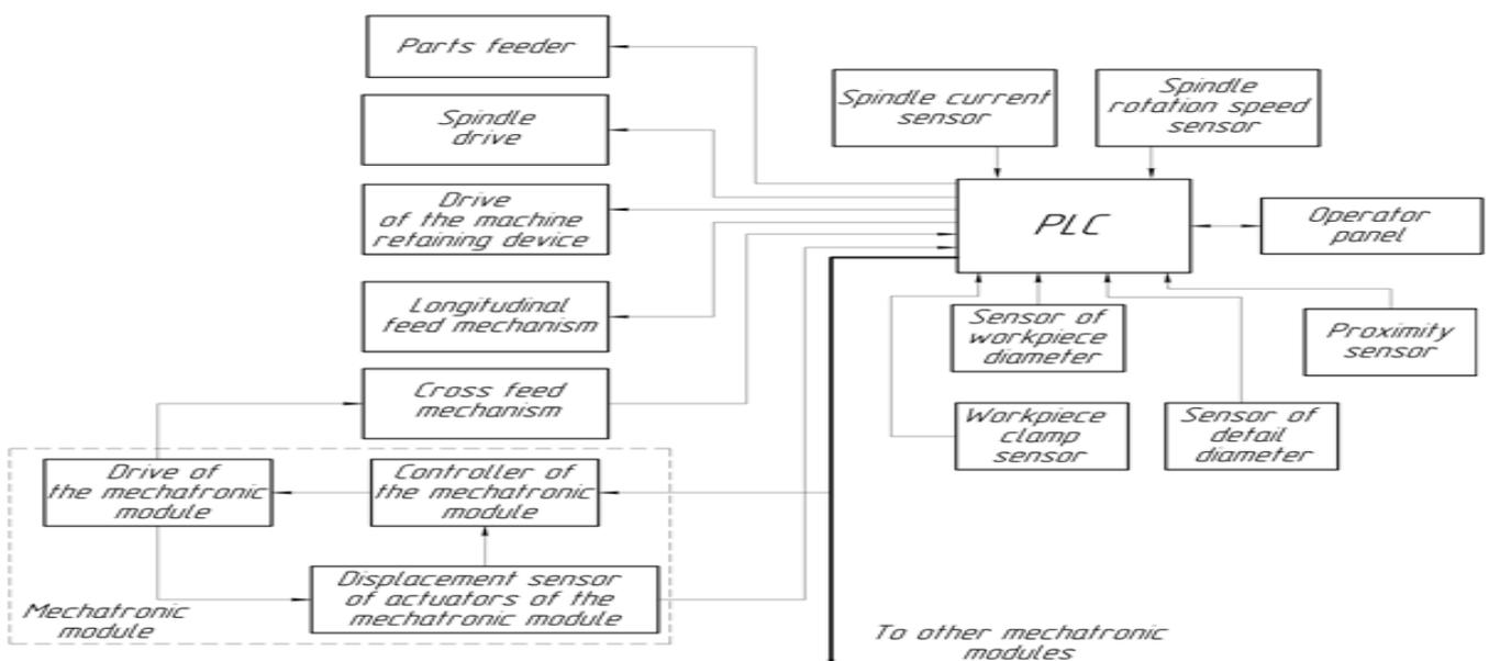
**Figure 1** - Block schematic diagram of swiss-type automated turning lathe control equipped with mechatronic modules.
