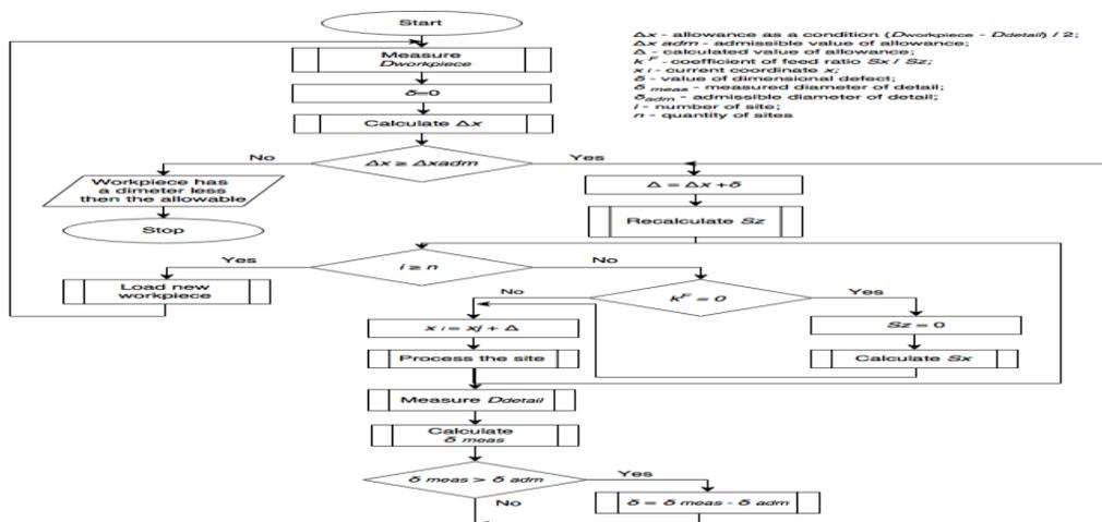
**Drawing 2** - Algorithmic diagram for the equipment control upon machining of workpieces.
