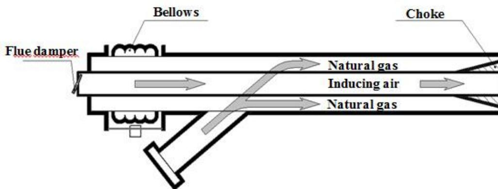
**Figure 2.** Schematic diagram of burner of GID type (two-circuit injection-diffusion gas burner)
