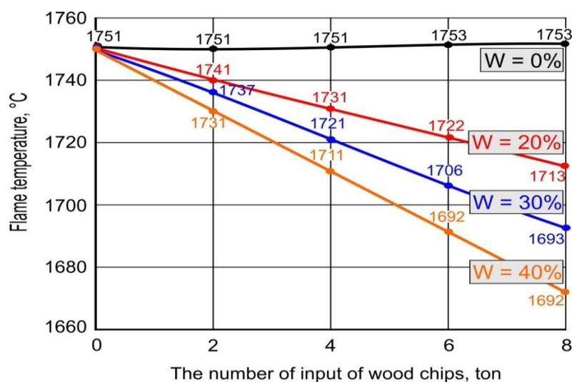
**Figure 3.** Impact of share of the input of wood chips on the flame temperature given its moisture content
