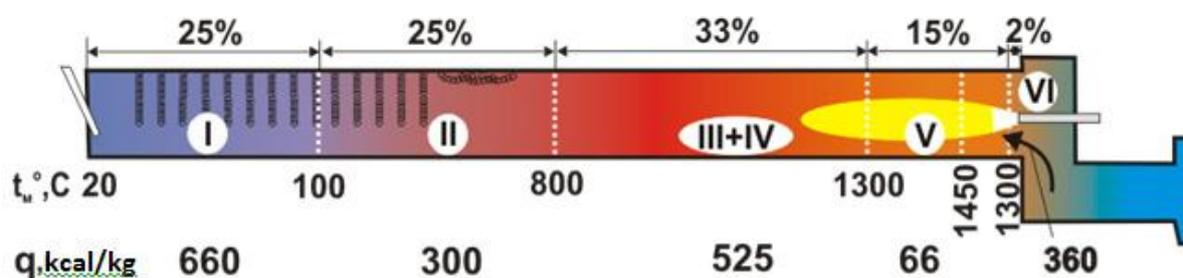
**Figure 1.** Process zones in wet process kiln and heat consumption in the zones.
