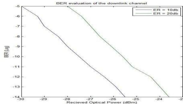
**Fig-8: BER Vs Downlink optical Power received.**
