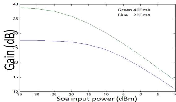
**Fig3 SOA Gain (dB) verses Input power (dBm)**
