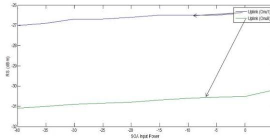
**Fig 6: Receiver Sensitivity of Uplink Channel.**
