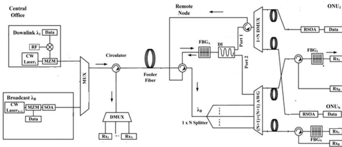
High insertion loss which is compensated by the gain of a semiconductor amplifier. An optical delay interferometer (DI) is used to separate all optical carriers and subcarriers of the SCM modulated downlink unicast signals, which is much more cost-effective than the method of dedicated filtering for each downlink unicast signal at each ONU.
