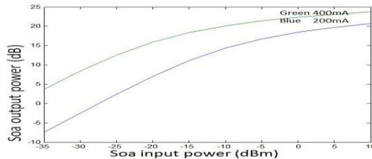
**Fig 2.SOA Input versus Output power (dBm).**
