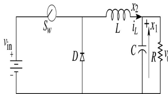
**Fig(1): Model of buck converter.**
