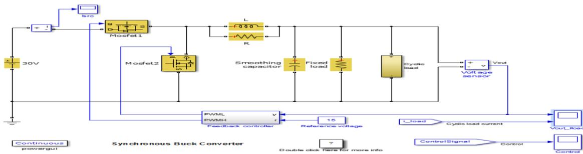
**Fig(4):Synchronous Buck Converter using PI controller**
