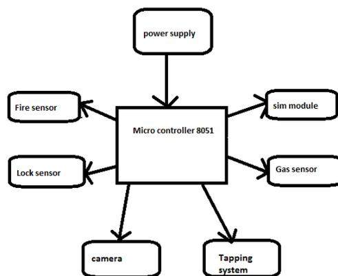
Fig:1-Block diagram for the proposed system.
