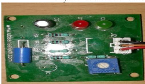
**Fig 3.3 Vibration sensor**
