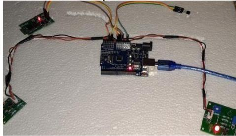
**Fig:5.1 Structural Health monitoring prototype**
