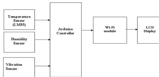
**Fig:1 Block Diagram III. Proposed Structural Health Monitoring.**
