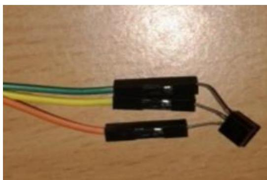
**Fig 2.5: Temperature sensor.**
