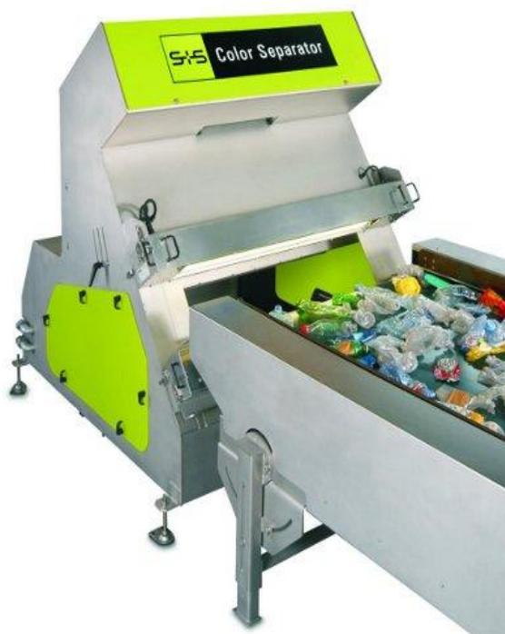
**Fig.a:** This machine sorts bottles and other containers made from different polymers prior to cleaning and shredding. It distinguishes between different polymers using a NIR (near infra-red) detector. This distinguishes between bonds in a molecule. There is also a separate detector which allows metals to be removed.
