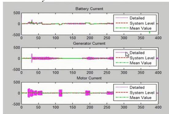
**Fig. 5(c). The current response of the system with respect to drive cycle.**
