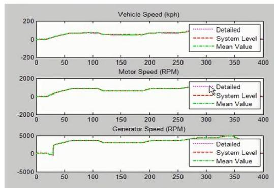
**Fig. 5(a). Speed response of the system with respect to drive cycle.**
