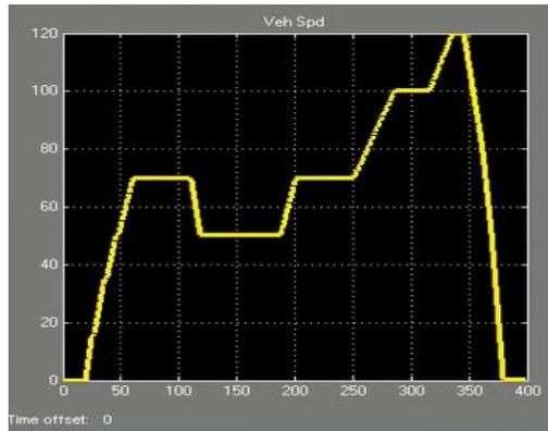
**Fig.5. Drive cycle of the hybrid vehicle.**
