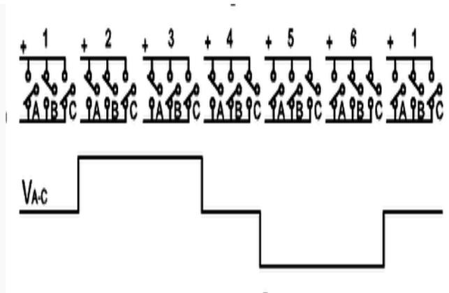
3-phase inverter switching circuit showing 6-step switching sequence and waveform of voltage between terminals A and C ( $2^3 - 2$  states)
