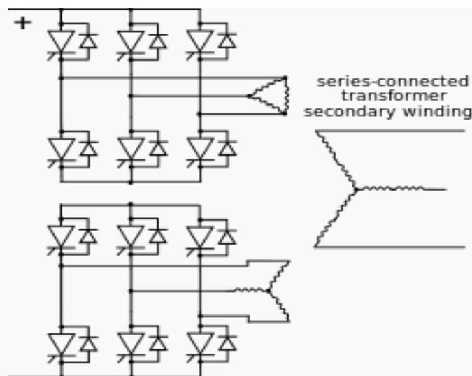
Fig 3. line-commutated inverter circuit
