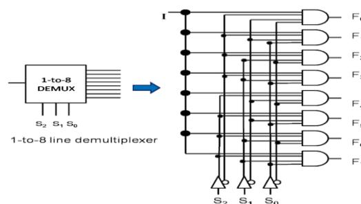
Fig 5.Demux circuit diagram.
