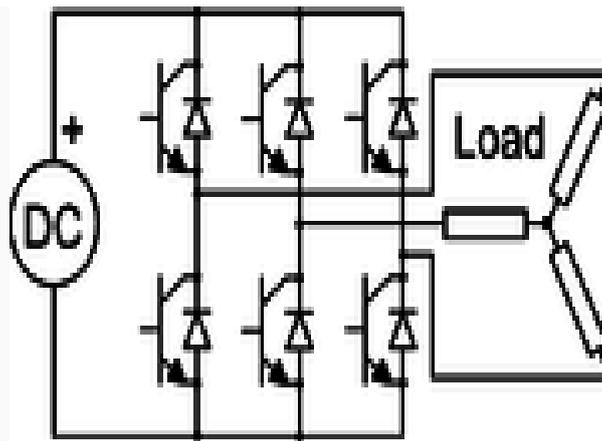
**Fig 2.three phase inverter**
