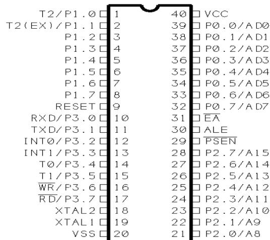
**Fig. 3 Pin Diagram of AT89S52.**
