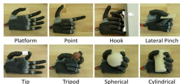
**Fig 1.17 Uses of Prosthetic Hand.**
