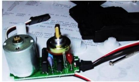
**Fig 1.7 Inside a Servo motor.**
