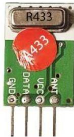
**Fig 1.10 RF 433 MHz Transmitter Module.**
