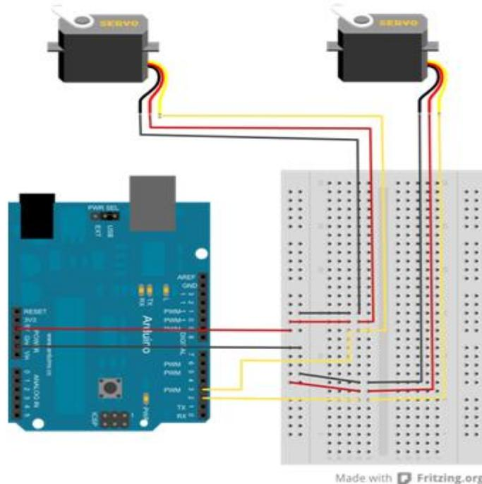
We use servos here to control the cameras position on the wheel chair handle. We had used Fritzingto simulate the circuit and used Arduino software for servos simulation.
