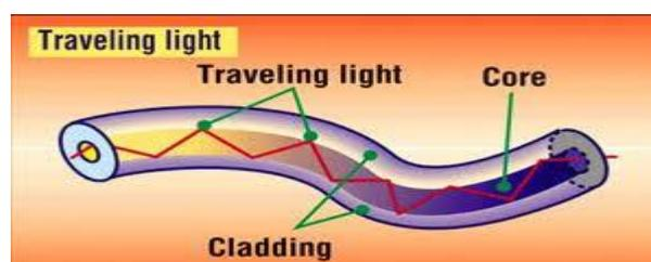
**Fig 4.1 structure of optical fiber.**
