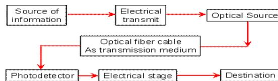
**Block Diagram of Optical Fiber Communication.**
