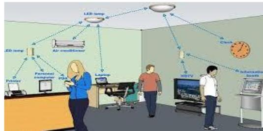
**Fig.2 Replacing Wi-Fi with Li-Fi (In the above figure the devices were accessed by Li-Fi).**
