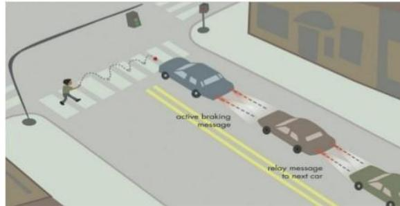
**Fig.3.4 vehicle to vehicle Li-Fi communications.**
