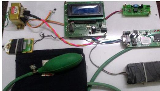
**Fig 1.5: Experimental setup of heart rate, body temperature, blood pressure and sweat sensors.**
