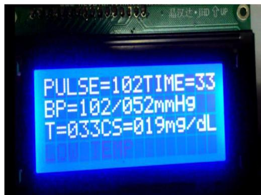
**Fig 1.6: Result for blood pressure and heart rate**
