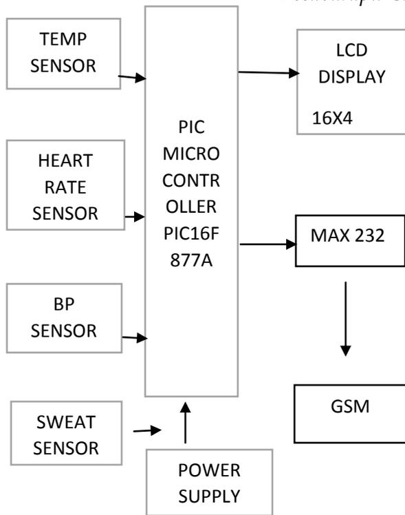
**Fig 1.1: Block diagram of proposed system.**
