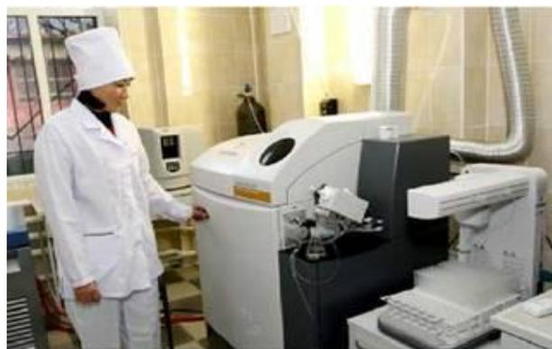
**Figure1-Inductively coupled plasma mass spectrometry with a quadrupole mass analyzer from Varian 820MS (USA).**
