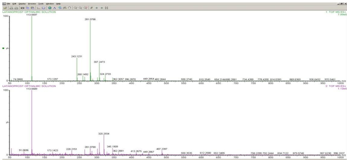
Figure -6a. ESI-MS<sup>E</sup> Spectrum at Low and High Collision Energy (impurity RRT 0.38).
