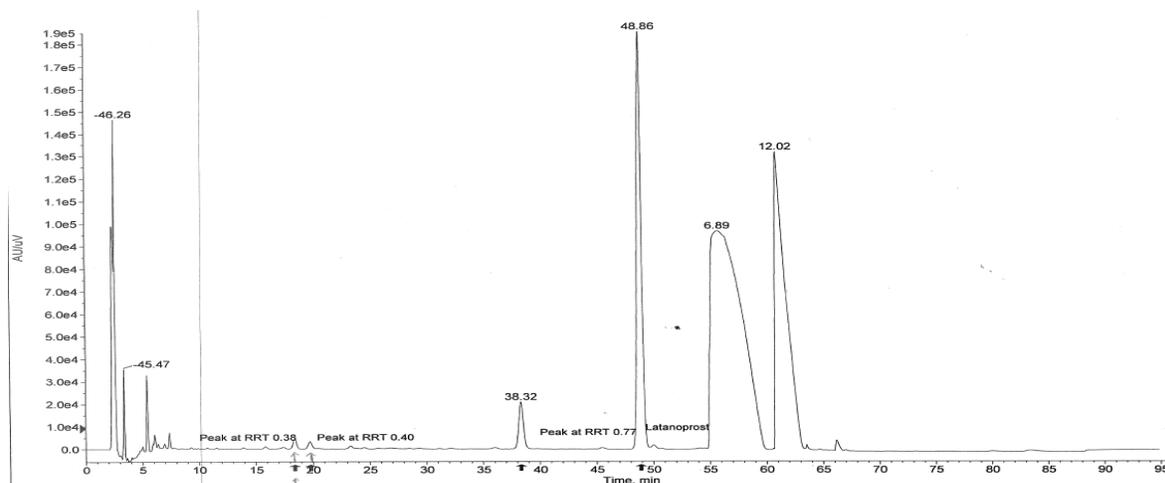
**Figure - 2. HPLC chromatogram of Latanoprost.**
