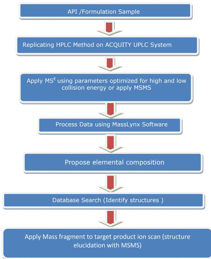
**Figure-4. Workflow for Impurity Identification in Formulation.**
