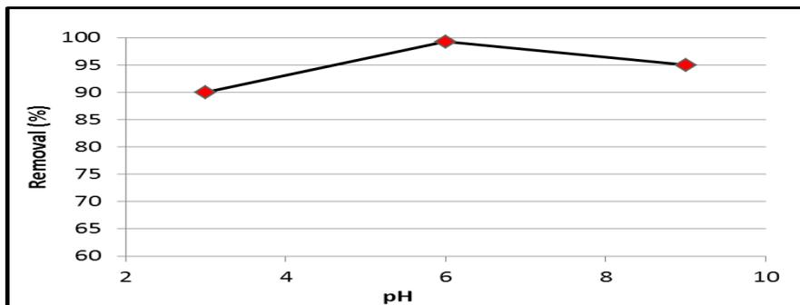
**Figure-4. The removal efficiency changes based on the pH (the optimum adsorbent level 2.5 gr and balance time of 2h and optimum adsorbate concentration of 10mg/l).**
