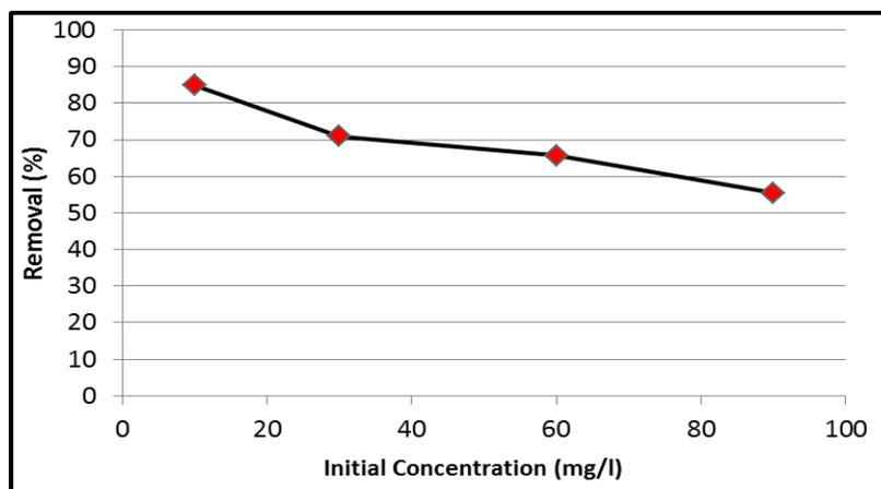
Figure-3. Removal efficiency in various cadmium concentration (the optimum adsorbent amount of 2.5 gr and balance time of 2hours).
