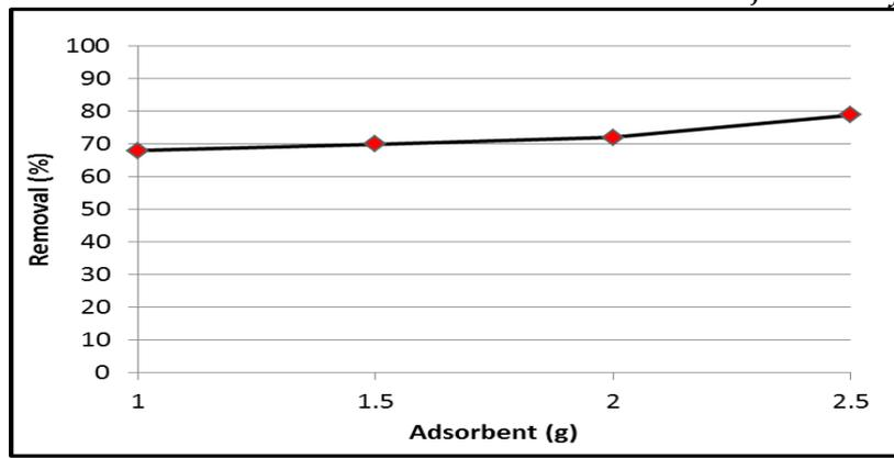
Figure-1. The removal efficiency based on the various adsorbent amounts.
