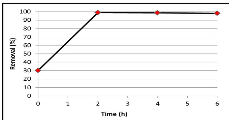
Figure-2. The removal efficiency in various time of initial concentration (30mg/l).
