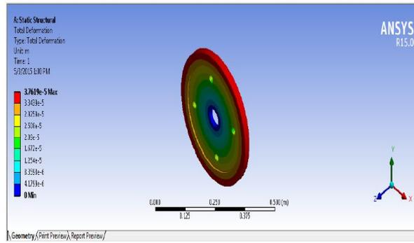
**Figure 3 Total Deformation.**
