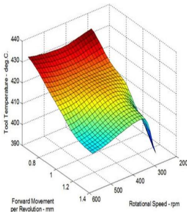
Figure-2. Model predicted tool temperature in a Friction Stir Welding tool during the welding of aerospace grade aluminium plates. Via the developed models the system can ‘map’ process conditions and internal process variables to the performance of the material. [24]
