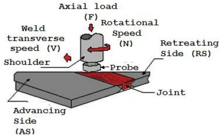
**Figure 1 Schematic illustration of Friction Stir Welding.**
