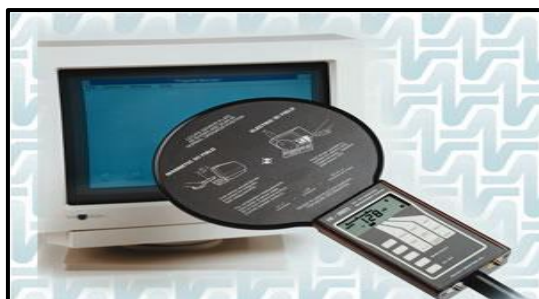
Figure-1. Portable device measuring electromagnetic field, Model HI-3603-VDT/VLF.
