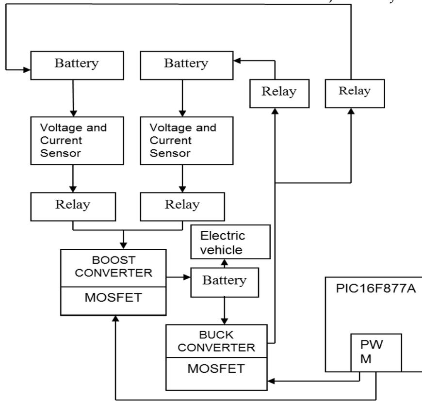
**Fig1. Block diagram of constant power load stabilization.**
