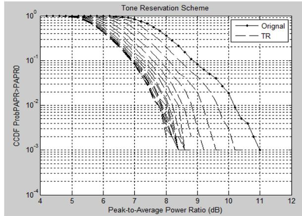
**Figure 2 PAPR Reduction using Tone Reservation Scheme for DSTBC MIMO-OFDM System.**
