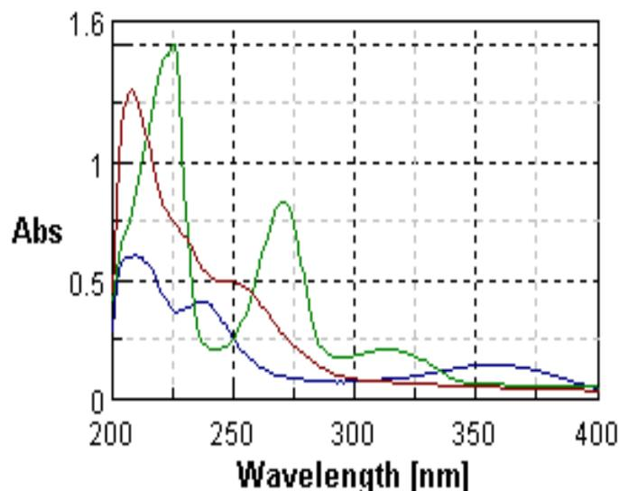
Figure 5 Overlain first order derivative spectra of VAL, AML and HCZ (10µg/ml)
